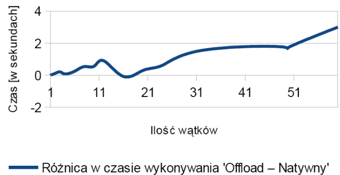
Fig. 3. Comparison of accelerations obtained on Intel Xeon Phi in offload mode and in native mode. Source: Own data.
